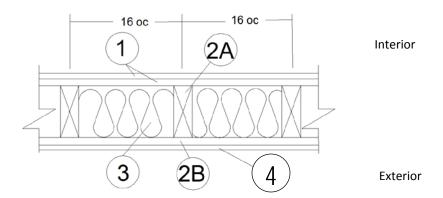
1. **GYPSUM BOARD (Interior):** Two layers USG Firecode® C Core, complying with ASTM C1396, or equivalent, min. 5/8 in. thick, 4 ft. wide applied vertically, fastened to framing. Face layer joints staggered with base layer and covered with paper tape and joint compound.
