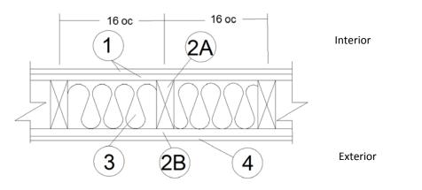
GYPSUM BOARD (Interior): Two layers USG Firecode<sup>®</sup> C Core, complying with ASTM C1396, or equivalent, min. 5/8 in. thick, 4 ft. wide applied vertically, fastened to framing. Face layer joints staggered with base layer and covered with paper tape and joint compound.
