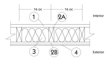
1. GYPSUM BOARD (Interior): One layer Type X, complying with ASTM C1396, min. 5/8 in. thick, 4 ft. wide applied vertically, fastened to framing. Joints covered with paper tape and joint compound. Fasteners covered with paper tape and joint compound. Min. #6 x1-5/8 in. long Type S or W screws, spaced max. 6 in. on center (oc).
